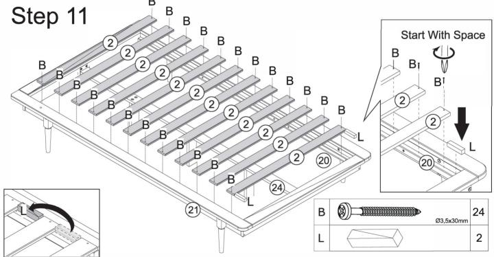
Place part 2 onto parts 20,21. Use part (L) to space part 2 from the end and secure with screw (B) using a Phillips head screwdriver.
