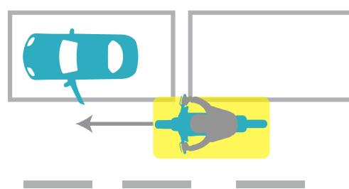
DOW is activated when under two conditions: when the engine is on and the hazards indicators are activated, and five minutes after stopping the engine. An audible tone will be heard, and the warning indicator lamp will flash with an object or vehicle is within the warning zone, or if there is a vehicle detected approaching at high speeds resulting in an impact of less than 2 seconds.
