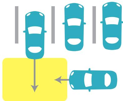
Rear Cross Traffic Alert helps you avoid accidents when driving in reverse, such as backing out of a parking spot. The system activates when you place your vehicle in 'reverse'. An audible tone will be heard and the corresponding warning indicator lamp will flash when a pedestrian or vehicle is detected, which would result in an impact of approximately 2 seconds. The system is capable of monitoring the rear cross traffic zones up to a 60 ft range.
