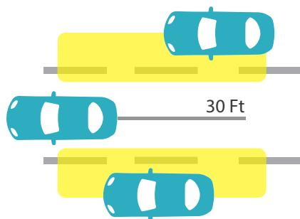
The system is automatically activated when the vehicle exceeds 15 MPH to alert you of vehicles in your side blind spot. The warning indicator lamps will illuminate when a vehicle is within the warning zone (75 Ft range in the lanes to the right and left of you), or if there is a vehicle detected approaching at high speeds resulting in an impact of less than 2 seconds. (ISO 17387 Type 3 compliant)
