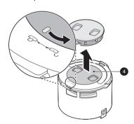
7 Press and lift the hook **5** up to remove the pre-filter **6**.
