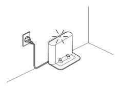
4 Wrap the unwanted length of power cable around the cord keeper to prevent the robot cleaner wheels from rolling over the cable.
