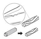
· Dust may build up at the brush inlet at the bottom of the brush. Periodically remove the buildup using another vacuum cleaner or a soft brush.
