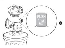
Remove any foreign substances on the rubber at the bottom of the dust bin.
