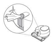
Turn the robot cleaner over and clean the cliff detection sensors 1 and the charging terminals 2 using a cotton swab or a soft cloth.
