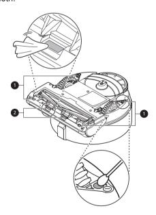
4 Clean the dust sensors on the robot cleaner using a soft cloth.
