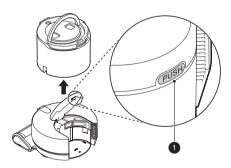
2 Press the dust bin release (PUSH) button 2 to open the dust bin cover and empty the dust
