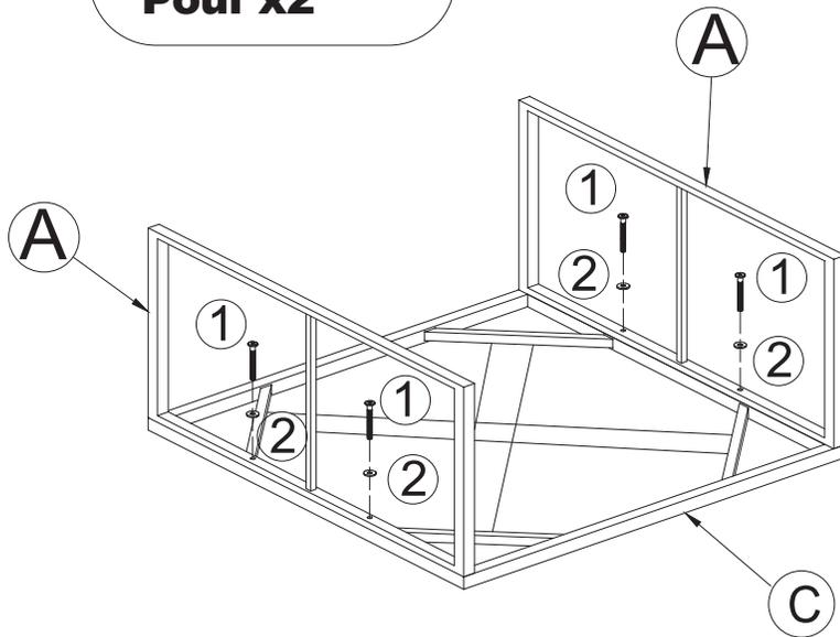
Please don't fasten the screw completely during assembly process. It will be likely to lead to an assembling problem that screw hole position is not aligned. You can fasten completely when all parts have been assembled.
