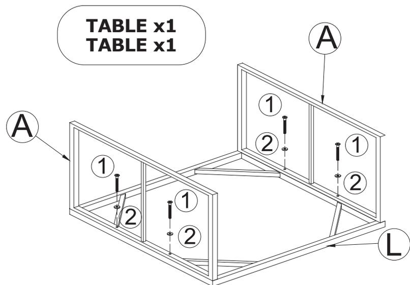
Please don't fasten the screw completely during assembly process. It will be likely to lead to an assembling problem that screw hole position is not aligned. You can fasten completely when all parts have been assembled.
