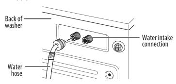
2 Turn the water on and check for leaks.
