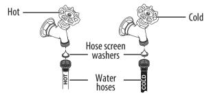
4 Place the unconnected end of the hoses into a bucket, then turn on the faucets connected to the water supply hoses for 10 or 15 seconds to remove any foreign substances. Turn off the faucets.
