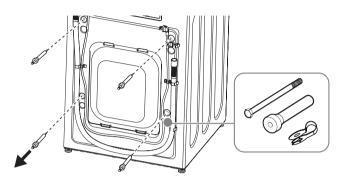
2 Insert the hole caps (attached next to the bolt holes on the back of the washer) into the bolt holes after the shipping bolts, spacers, and retainers have been removed.
