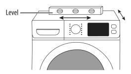
3 Loosen the lock nut on the bottom of your washer, pull the leg down until it touches the floor, then tighten the nut. Extend the feet only as much as is necessary. If the feet are extended too much, your washer may vibrate.
