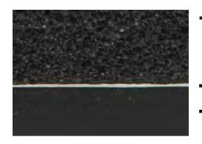
Acoustic foam outer layer that absorbs and diffuses high frequency sounds, acts as a thermal barrier, and absorbs soundwaves that are otherwise trapped inside the empty space behind door panels.
