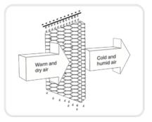
The evaporative air cooler can also be used to humidify dry environments (during cool weather). To be used for humidification the windows and doors should be closed to allow the humidified air to accumulate. The evaporative air cooler is not an air conditioner as it does not use a compressor or refrigerant. It should not be expected to cool as effectively as a refrigerated air conditioner.
