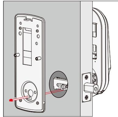
**4.2:** Place the mounting plate on the interior side of the door. Guide the cable to the opening ear on the side of mounting plate and make sure the torque blade is at the center of the mounting plate.
