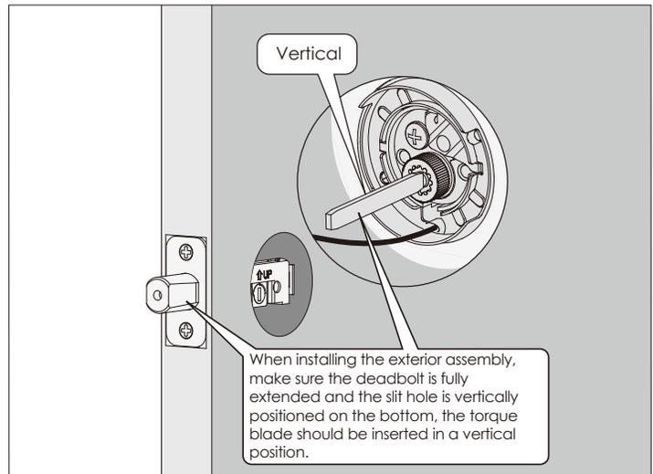
**3.3:** Place the exterior assembly on the door by inserting the torque blade on a vertical position to the deadbolt slit hole + and guide the cable under the deadbolt. Secure and fastened with the adhesive strips.
