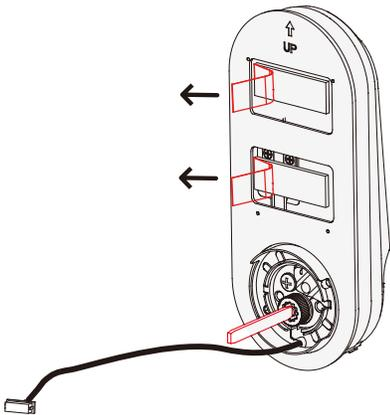
**3.2:** Before placing the exterior assembly on the door, make sure the torque blade is in vertical position and the deadbolt is extended.
