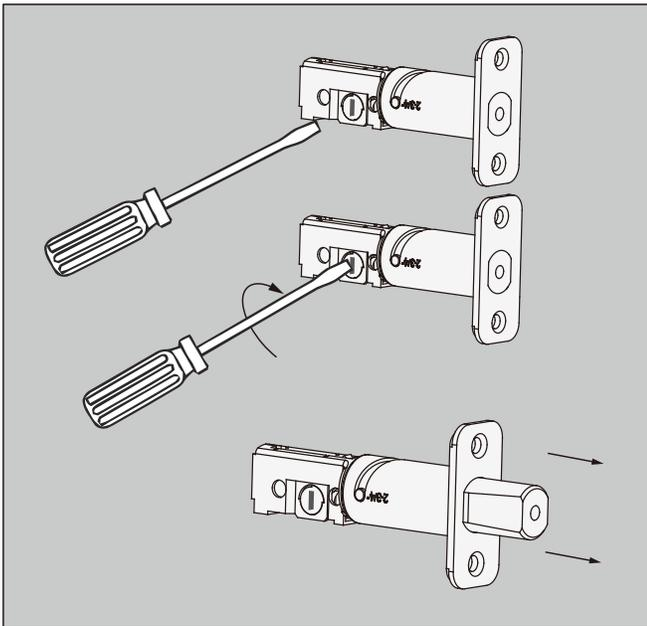
**2.3:** Insert the Deadbolt to the edge door hole, make sure that its right side up and the slit hole is in vertical position, then fastened with 2 screws (K)
