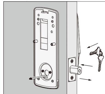
**4.4:** Before installing the interior assembly, use the physical key and try to unlock/lock to check if the deadbolt is moving and not stuck. Do not forget to take out the key before proceeding to next steps.
