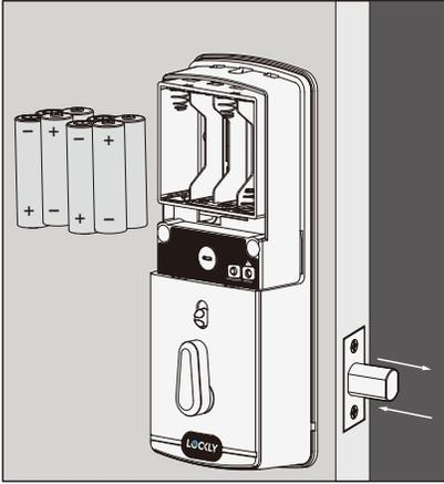
**5.1:** First install 3 of the 4 batteries. Before installing the last battery, press and hold the PROGRAM button
