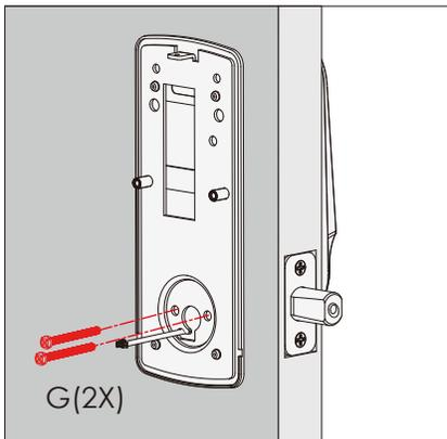
**4.3:** Without using any tools, insert 2 screws (G) on the side of the torque blade. By using hand carefully, turn the screws clockwise to catch the thread, then counter clockwise to make sure they are not cross threaded and turns smoothly. Make five turns before using a screw driver to tighten the screws until the mounting plate is securely placed to the door.
