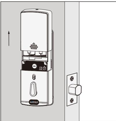
**5.2:** After you checked that the lock manually lock and unlock and deadbolt moves smoothly, Install the battery cover with screw (H) and fastened.
