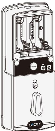
**4.7:** Place the interior assembly against the mounting plate and make sure the torque blade is inserted to the thumb turn shaft.
