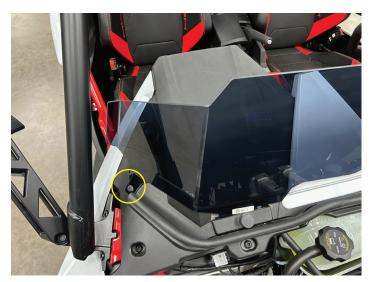
Remove passenger mirror bolts or cage bolts using an 8mm Allen wrench. Repeat on driver side.
