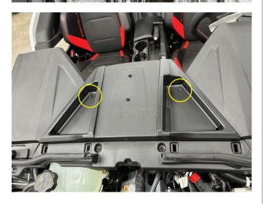
If equiped with a ROPs, lift ROPs up to provide clearance. Lift dash upward above instrument cluster and remove. If equipped with OEM tweeters, slide dash forward and disconnect from harness on both sides.
