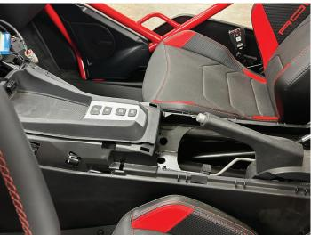
• Reinstall rear cupholder / arm rest into the center console.
