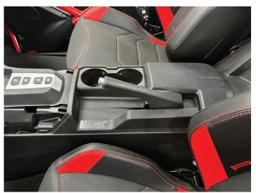
• Unclip rear edge of shifter console, slide rearward and set to the side.
