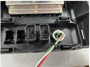
Install switches, switch trim panel and GMR-7 radio. Flip dash over and secure GMR-7 with four M4 washers and M4 x 10mm Phillips screws.
