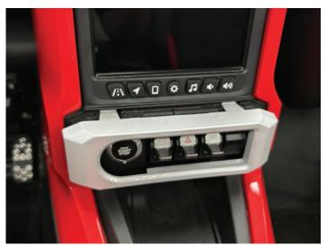
Remove two T40 Torx screws and two push-pin rivets from either side of top center dash. Unclip center dash by cup holder and pull to rear of vehicle to remove.
