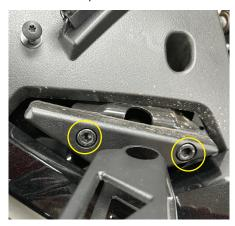
If equipped remove upper center painted panels by gently unclipping panel towards the motor and lifting up.
