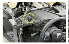
• Pull out and unclip switch trim on center console.
