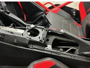
Route antenna wire toward rear of vehicle zip tieing along OEM wiring on driver side center console.
