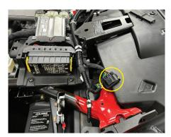
Unclip front edge of cupholder and rear center console. Remove from vehicle
