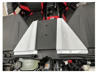
On driver side painted dash panel remove two plastic push-pin rivets and two T25 Torx screws and gently lift panel up. Repeat on passenger side.
