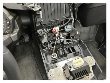
Remove all switches from the dash, Note locations the switches are being removed from.
