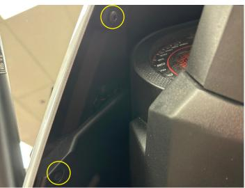
• On driver side remove four T40 Torx screws from the front of the dash.
