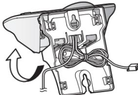
5 Mount the unit on a wall then slide down to secure in place.
