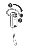
3. Attach a earhook, and then a suitable earbud to the headset until they fit into place. To wear on the right ear:
