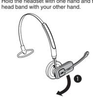
2. Rotate the headset to vertical direction and the pull the headset until it separates form the head band.
