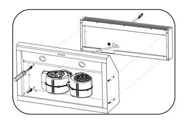
6.The reserved size on both sides of the circulation cover and cabinet shall not be less than 1/16 "(6.1), and the reserved size between the top of the Recirculating Kit and the bottom of the cabinet shall not be less than 4-1/8" (6.2). Make sure the filter is securely engaged after assembly.
