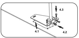
5.Put the Recirculating Kit on corresponding position behind or on the top at range hood, and secure it to the range hood with the matching screw.
