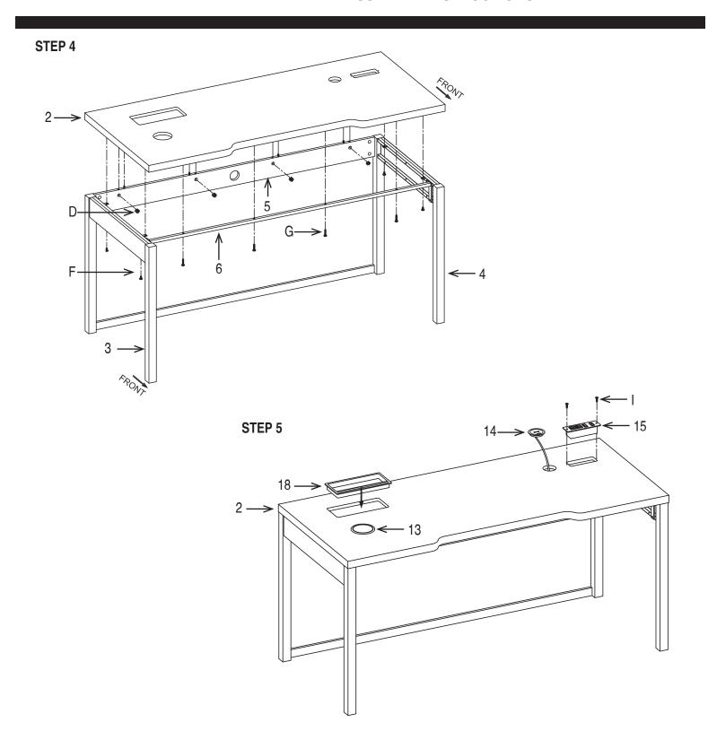
STEP 4 Attach Desk Top (2) to assembly. Secure Desk Top (2) using four Allen Bolts (F) for Side Frames (3 & 4), four Cam Nuts (D) for Back Panel (5) and four Allen Bolts (G) for Middle Front Crossbar (6). APPLY FIRM PRESSURE TO ALIGN & FULLY TIGHTEN ALL CAM NUTS (D) AND ALLEN BOLTS (F & G).
