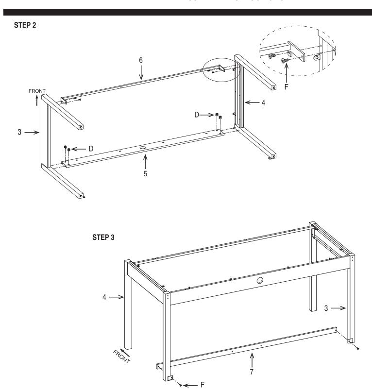
STEP 2 Attach Back Panel (5) between Side Frames (3 & 4) and secure using four Cam Nuts (D). FULLY TIGHTEN ALL CAM NUTS (D). Attach Middle Front Crossbar (6) between Side Frames (3 & 4). and secure using four Allen Bolts (F). DO NOT FULLY TIGHTEN ALLEN BOLTS (F). STEP 3 Carefully turn assembly to the upright position. Attach Rear Lower Crossbar (7) between Side Frames (3 & 4) and secure using two Allen Bolts (F). DO NOT FULLY TIGHTEN ALLEN BOLTS (F).
