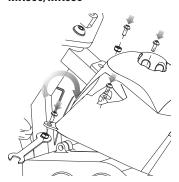
**10** Using a 5 mm Allen wrench and a 10 mm wrench, reinstall the four (4) Allen bolts that hold the fairing in place. The two (2) screws at the bottom are held by 10 mm locknuts.
