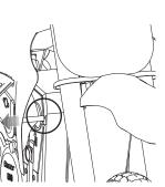
**3** Pull the left and right leafboards apart to remove the positioning column from the battery box and using a 4 mm Allen wrench, remove the two (2) bolts from the top of the battery cover and three (3) more on each side and remove the covers.
