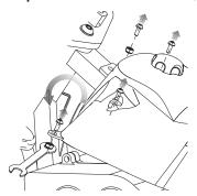
1 Using a 5 mm Allen wrench and a 10 mm wrench, remove the four (4) Allen bolts that hold the fairing in place. The two (2) screws at the bottom are held by 10 mm locknuts.
