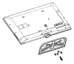
3 Remove the four screws that secure the stand column, then remove the column.
