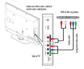
3 Connect an audio cable to the L/R (audio in) jacks on the side of your TV and to the L/R AUDIO OUT jacks on the component video device.
