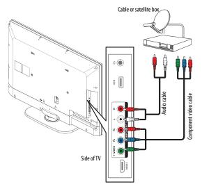
4 Connect an audio cable (included) to the L and R audio jacks on the side of your TV and to the audio out jack on the cable or satellite TV box.
