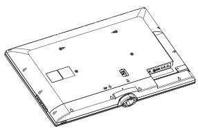
2 Secure the stand to the TV with the four provided screws.
