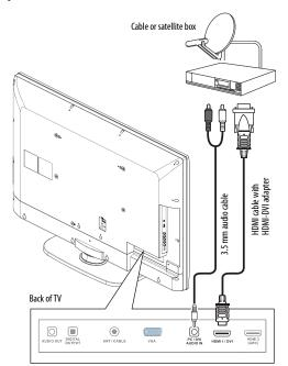
5 Connect a 3.5 mm audio cable (not included) to the PC/DVI AUDIO IN jack on the back of your TV and to the AUDIO OUT jack on the cable or satellite box.
