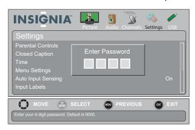
**4** Press the number buttons to enter the four-digit password. The *SETTINGS-Parental Controls* menu opens.
