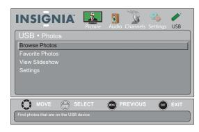
4 Press ▲ or ▼ to highlight Browse Photos, then press ENTER. The screen displays folder names and photo files stored on the USB flash drive in a thumbnail index with the first photo or folder highlighted. A control bar appears at the bottom of the screen.
