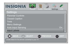
3 Press ▲ or ▼ to highlight Input Labels, then press ENTER. The SETTINGS-Input Labels screen opens with the input source field highlighted.
