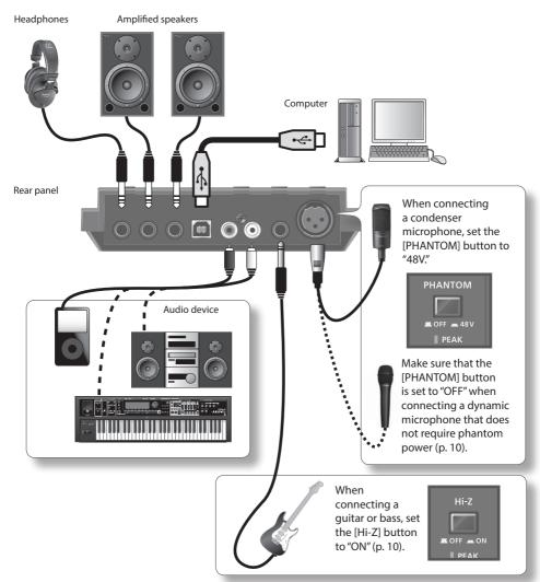
Use the corresponding knob ([INPUT 1 (MIC)], [INPUT 2 (GUITAR)], or [INPUT 3 (AUX)]) to adjust the volume of the microphone, guitar, or audio device so its PEAK indicator does not light.
