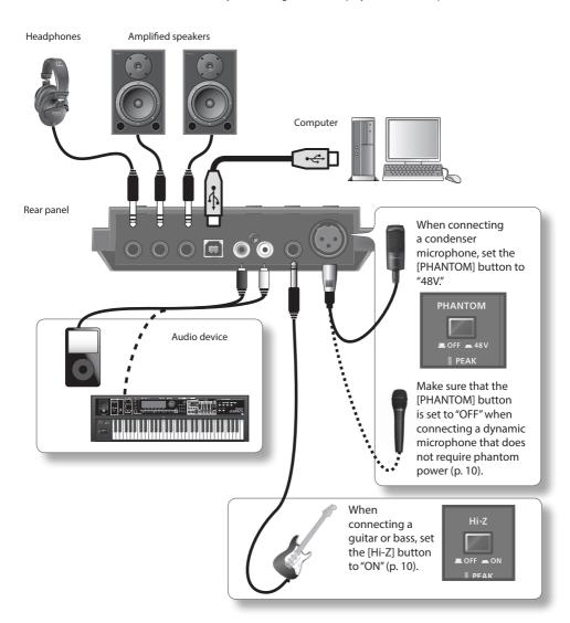
Use the corresponding knob ([INPUT 1 (MIC)], [INPUT 2 (GUITAR)], or [INPUT 3 (AUX)]) to adjust the volume of the microphone, guitar, or audio device so its PEAK indicator does not light.
