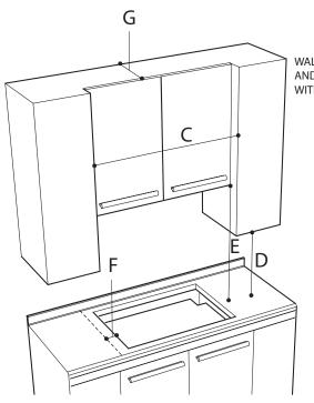
WALL COVERING CABINETS, AND COUNTERTOP MUST WITHSTAND HEAT UP TO 93° C (200° F)
