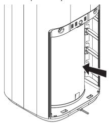
5 Insert the bottom of the filter cover into the purifier housing, then press the top of the cover to snap it into place.
