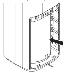
6 Insert the bottom of the filter cover into the purifier housing, then press the top of the cover forward to snap it into place.
