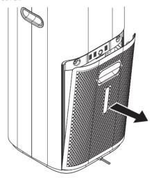
3 Pull the tabs on the top and bottom of the filter to remove it.
