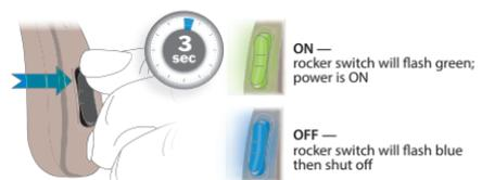
To turn ON or OFF, press and hold the **upper portion** of the rocker switch until you hear a beep (approx. 3 seconds) then release. While you are holding the rocker switch, it will turn green. The green light will turn off once the amplifier is ON.
