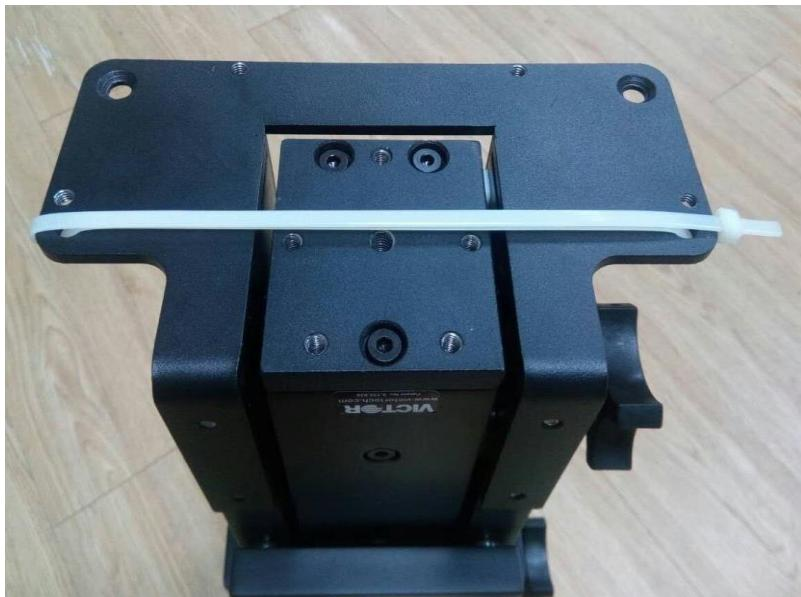
The Retention Straps prevent the Tower from movement during shipment. Remove before assembly.
