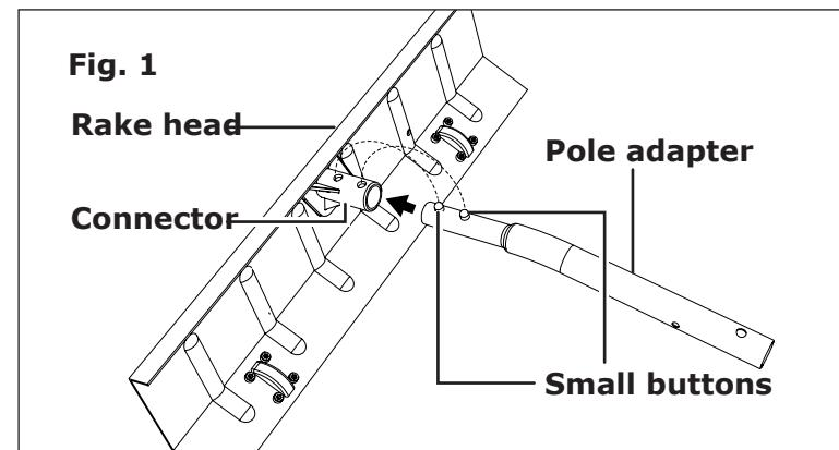
1. Depress the small buttons on the pole adapter and insert the pole adapter into the connector on the back of the roof rake head. Push firmly until the two small buttons pop up in the holes on the connector (Fig. 1).
