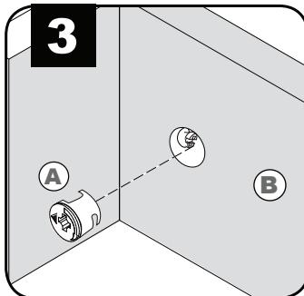
Insert Cam into side panel **B** Making sure **◀** points towards face panel **A**.
