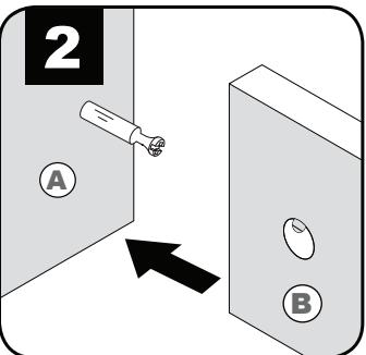
Push panels **A & B** together to insert spread bolt into cam hole.
