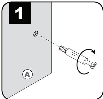
Screw the interlock bolt into the panel face **A**.
