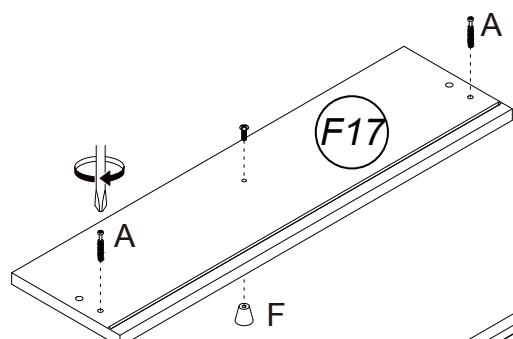
**LOCK** cam by turning 180° clockwise with a screwdriver.
