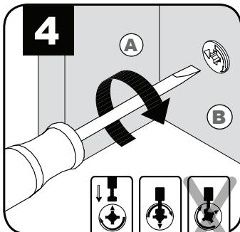
**LOCK** cam by turning 180° clockwise with a screwdriver.
