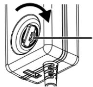
Knob options: 3V, 4.5V, 5V, 6V, 7.5V, 9V, 12V, 13.5V, 15V, 19.5V and 24V
