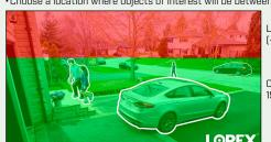
Angle the camera between 30~60° down from the level position.
