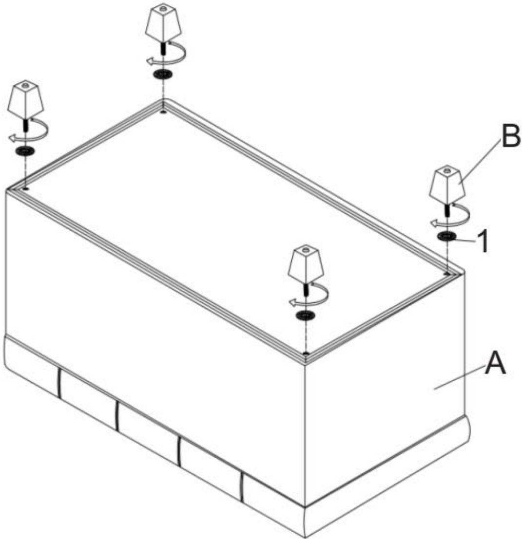
Place the Ottoman (A) on its back on a flat smooth surface. Attach the Feet (B) with Washer (1) to each corner.
