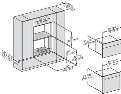
H 6x60 B/BP, DGC 686x AM, EBA 6808; H 6x70 BM, DGC 676x, DGC7xxx, H7xxxBP, EBA7868 Installation drawing, Flush inset, NA
