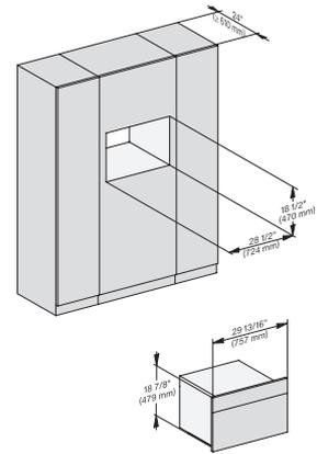
installation 30 inch Proud BM30, installation drawing, NA
