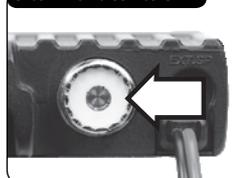
4. Make certain the antenna is properly assembled and connected. If you are unable to correct the problem, refer to product service on page 14 for the correct procedure for warranty and post-warranty service from Cobra.
