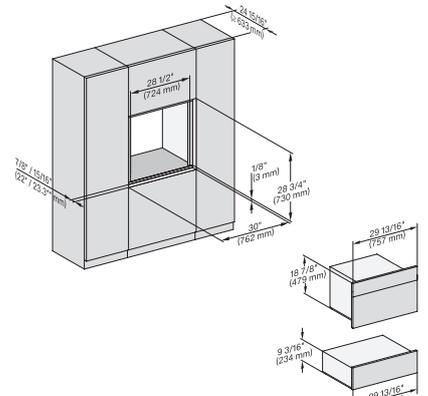
H 6x70 BM, ESW 6x85, DGC7x7x, H7x7x, Exx7x70 Fitting Combi, Installation drawing, Flush inset, NA
