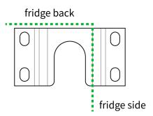
4. While the brackets are in position on the floor, mark the position of all 4 holes on each bracket. Before drilling any holes, double check all measurements and place the fridge near the brackets to check your accuracy. Bracket openings should line up with the adjustable feet on the back of the unit. Use a 5/16 drill bit to make holes for the plastic anchors. Insert the plastic anchors.
