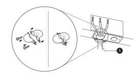
For conduit installations, insert the conduit strain relief in the 1 1/8 in. (2.8 cm) conduit hole. Then install the conduit through the body of the strain relief and fasten the strain relief with its ring.
