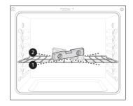
**2** If the level doesn't show that the rack is level, adjust the leveling legs with a wrench.
