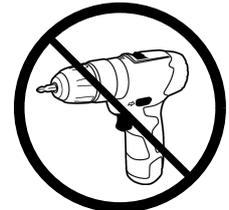
**Note:** Do not assemble using power tools. This can cause the bolts to be overtightened
