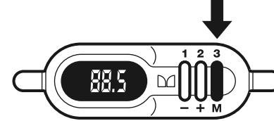
2. Press buttons 1 or 2 (also identified as '-' and '+') to scroll FM radio frequencies up or down.
