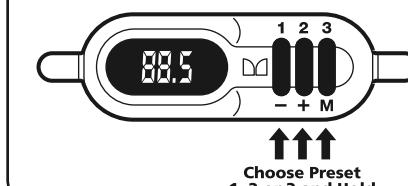
4. After your station is set, the unit will automatically go back to its default 'Preset' memory mode, where pressing the 1-3 buttons recall your default preset stations. To change presets, repeat steps 1 through 3.
