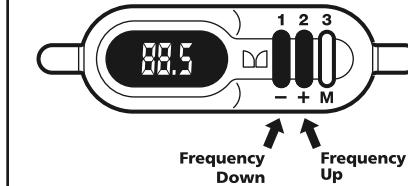
3. Once you've selected a station, press and hold any one of the three buttons for one second to set that station into memory and exit station selection mode. Your selection will be confirmed in the display as 1, 2 or 3.
