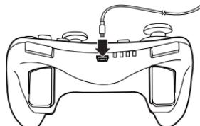
**IMPORTANT:** Make sure that the min-USB plug is aligned correctly with the port before inserting into the plug to avoid damaging either the port or the plug.
