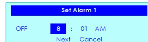
Press ▶ (SEEK UP) or ▶ (SEEK DOWN) to move the highlight to one of the options: ON/OFF, HOURS, MINUTES, or AM/PM.
