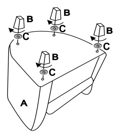
Place Chair (A) on its back on a flat smooth surface. Attach Feet (B) with Washers (C) to Chair (A).
