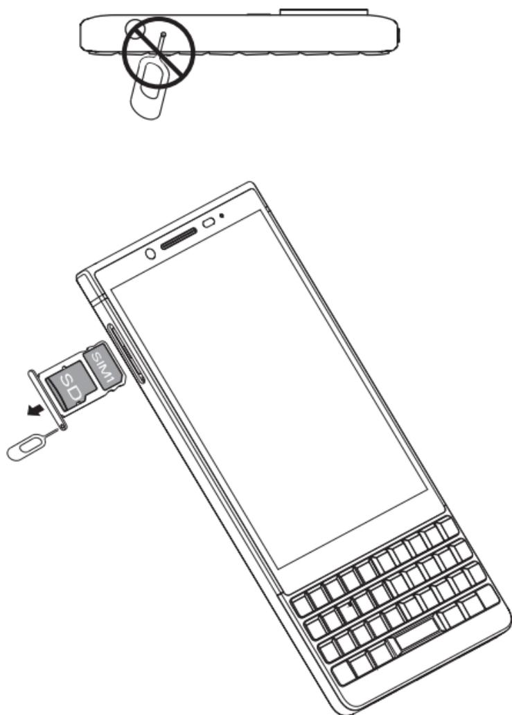
1. Insert the SIM tool (included) to where illustration shown above.
