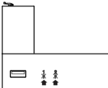
**6** When the battery pack is fully charged, slide the locking switch up to unlock.
