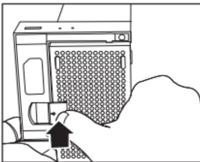
**4** Gently press the Side Dock Charging Station against the Xbox Series S to assure there is solid contact between the mounting pad and the console.
