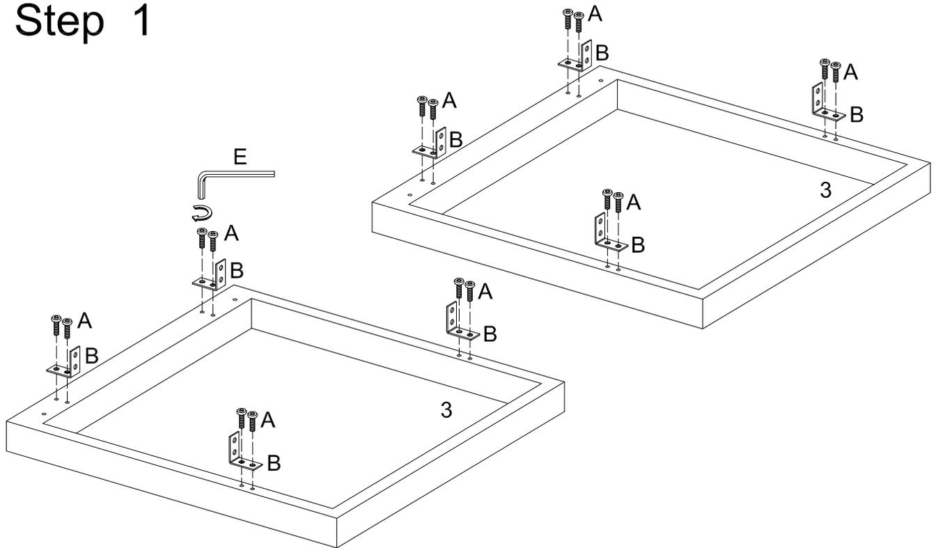
Place the Metal Frames (3) on the flat Surface, attached the L-shape connector (B) with the Bolts (A) and Wrench (E) as per diagram.
