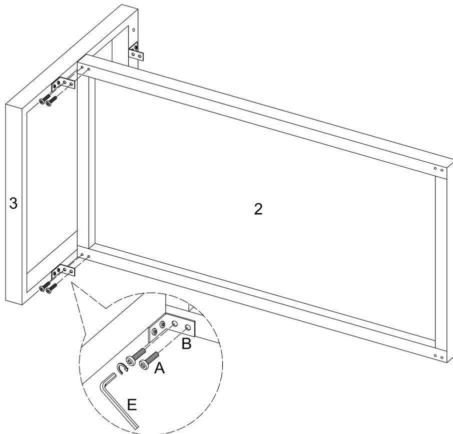
Attach the Lower Wooden Panel (2) to the Metal Frame (3) with Bolts (A), L-Shape Connector (B) and Wrench (E) for one side.
