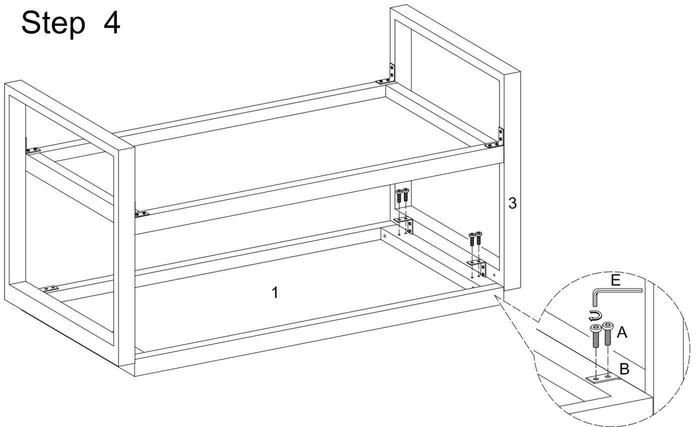
Up side down the Metal Frame (3) and the Wooden Panel (1) on a flat surface, Secure the wooden panel with the Bolts (A), the L-Shape Connector (B) and the Wrench (E).
