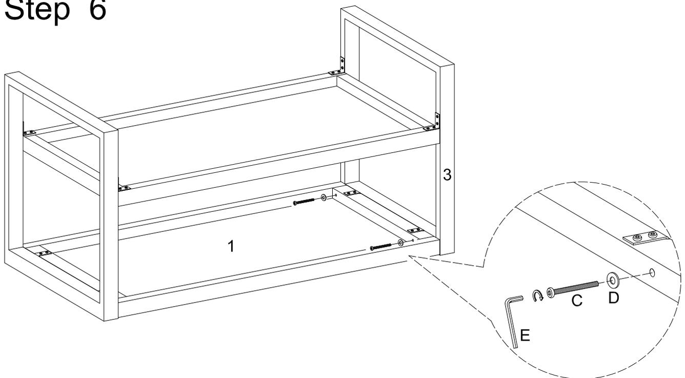
Use Washer (D), Bolts (C) and Wrench (E) to secure the Wooden Panel (1) to the Metal Frame (3).
