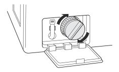
Close the drain pump filter cover.
