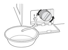
Clean the pump filter and opening.
