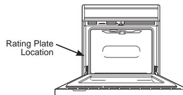
a circuit breaker or fuse having amperage as noted on rating plate. (Rating plate is located on front frame.) We recommend you have the electrical wiring and hookup of your oven done by a qualified electrician. After installation, have the electrician show you where your main oven disconnect is located.
