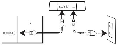
LED will pulse while connecting and then be solid when connections are confirmed
