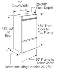
\* Shipping height. The refrigerator can be adjusted to fit into a cutout that is 84-1/2" max. height. Note that the top case trim at the front is 1/2" higher and will overlap upper cabinetry or soffit. Use leveling legs and wheels for a maximum 1" height adjustment.
