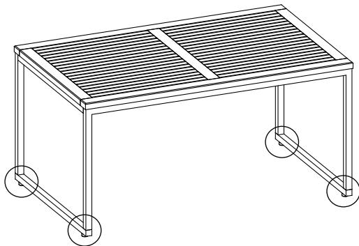
EN: The foot pads can be adjusted to fit uneven floors.
