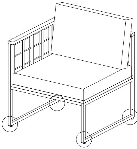
EN: The foot pads can be adjusted to fit uneven floors.
