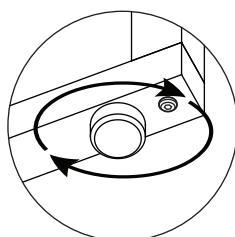
EN: The foot pads can be adjusted to fit uneven floors.
