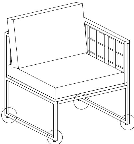
EN: The foot pads can be adjusted to fit uneven floors.
