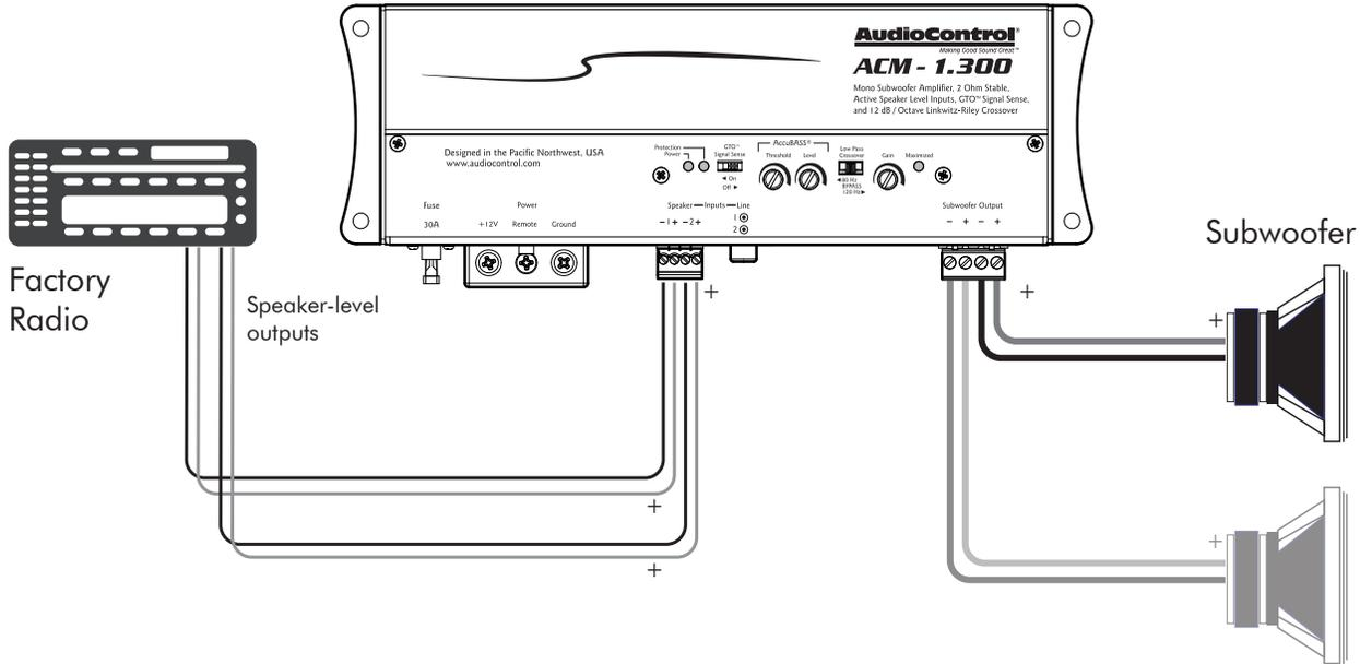
If two subwoofers are connected like this, they are in parallel, and the impedance of each subwoofer must be 4 Ohms or greater.
