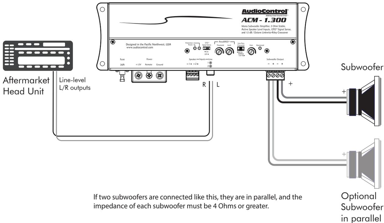
If two subwoofers are connected like this, they are in parallel, and the impedance of each subwoofer must be 4 Ohms or greater.
