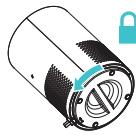
5. To lock the base cover back in place, align the locking notches, grip the twist handle, and firmly turn counter-clockwise until it clicks into locking place.
