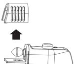
3 Unscrew and remove the old light bulb.
