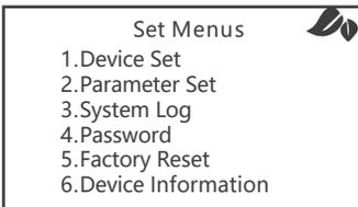
Use the UP and DOWN buttons then press OK button to enter the desired setting.
