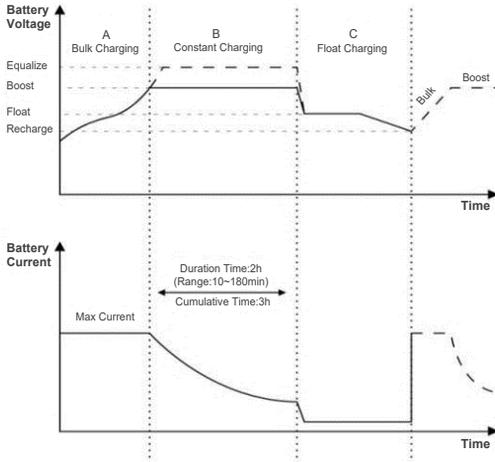
**Bulk Charge:** This algorithm is used for day to day charging. It uses 100% of available solar power to recharge the battery and is equivalent to constant current. In this stage the battery voltage has not yet reached constant voltage (Equalize or Boost), the controller operates in constant current mode, delivering its maximum current to the batteries (MPPT Charging).
