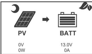
Displays solar panels Voltage and Wattage production on left side of screen. Shows Voltage and Amperage being sent to the battery on the right side of the screen
