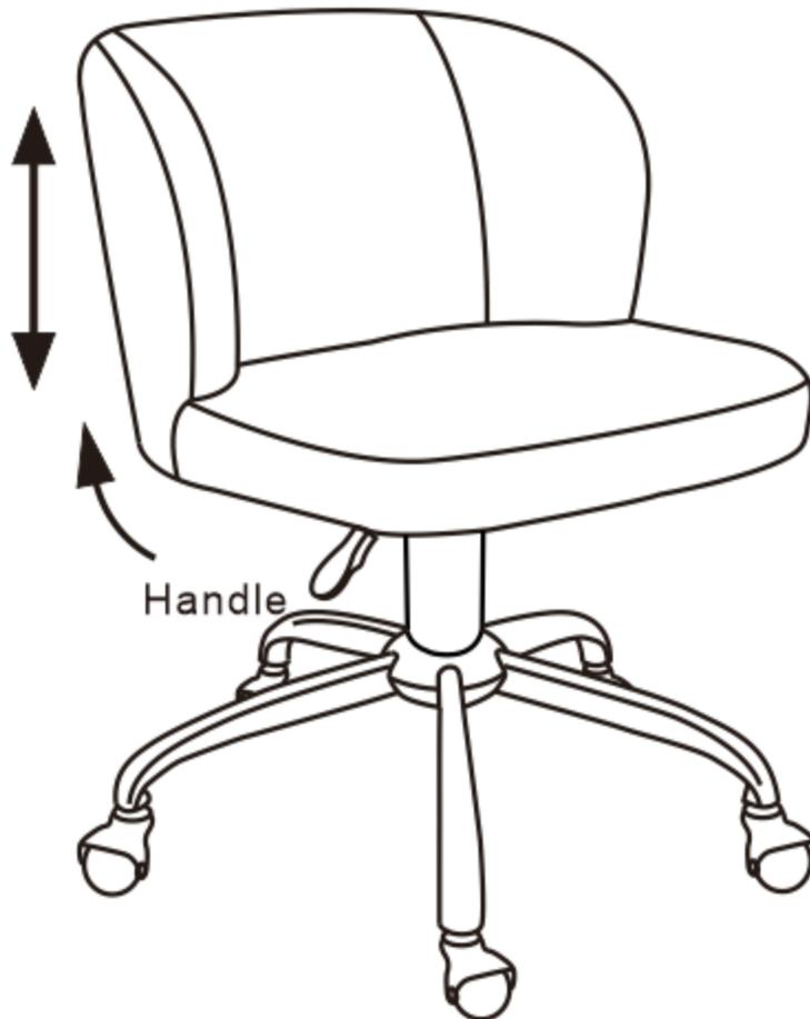
To raise the seat, lift your weight off the seat and reach underneath the right side of the Chair to lift the handle up slowly with a clockwise twisting motion to allow the Chair to rise to desired height.
