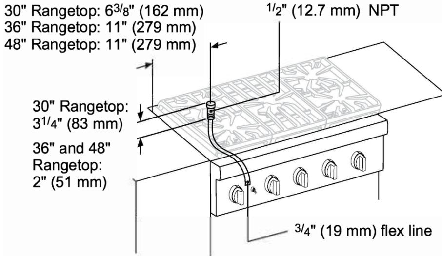
A manual valve must be installed to the appliance, in an accessible location from the front, for the purpose of shutting off the gas supply.
