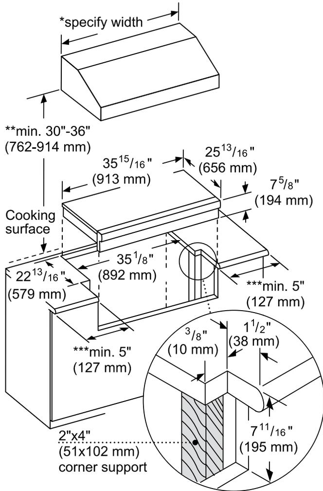
\*\* 36" minimum clearance from cooking surface to combustible surfaces.
